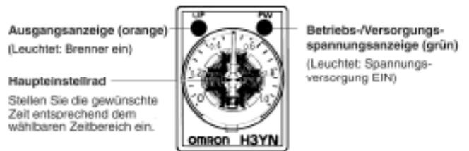
Output display (orange) (lights up: burner on)      Operational / supply voltage display (green) (lights up: voltage supply ON)
