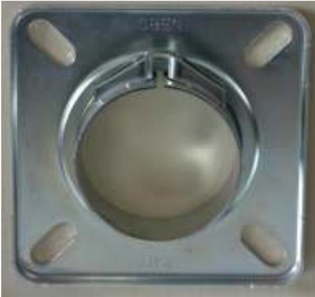
The sliding flange supplied with the equipment is used to affix the oil burner to the boiler by means of four bolts for attachment to the boiler plate. The jam-fit sliding flange facilitates insertion of the fire tube into the combustion chamber so as to meet the requirements of the specific boiler unit.
